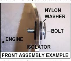
Carefully hold the Skid Plate up to the frame. Thread the 6mm bolt, with washer, into the the rear mount 2-3 turns. Thread the two RIMS bolts in 2-3 turns.
